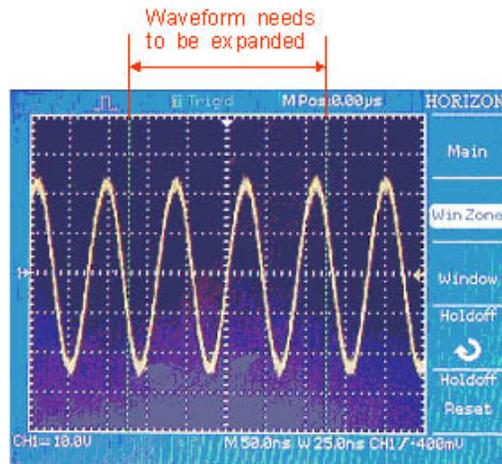
Figure 3-19 Window setup
