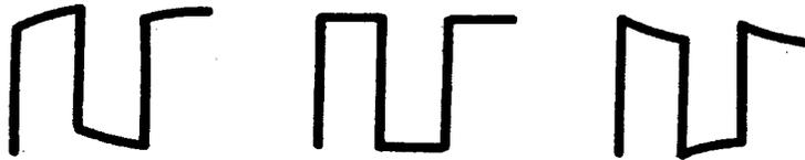
4. If necessary, use a non-metallic tool to adjust the trimmer capacitor on the probe for to resemble the Correctly Compensated wave shape as much as possible.
